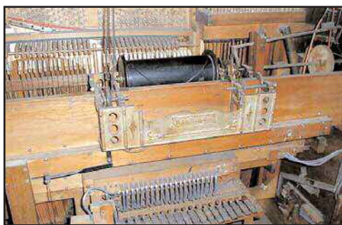
Figure 21. The last known CB&G Soleil IIa orchestrion reveals the construction of the firm’s roll frame and associated pneumatic system. The roll frame casting left no doubt about the inventor’s name and the fact that the design was protected. Image courtesy Bill Soper.
