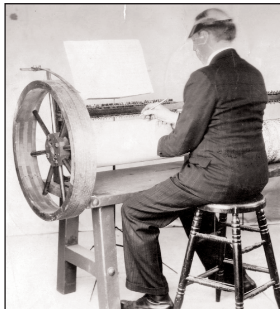
Figure 53. Among the exhibits in the "Mangels museum" in Coney Island was this vintage cylinder arranging machine from the Dentzel shop, the measuring wheel for which suggests Bacigalupo origin and use. Author's collection.
