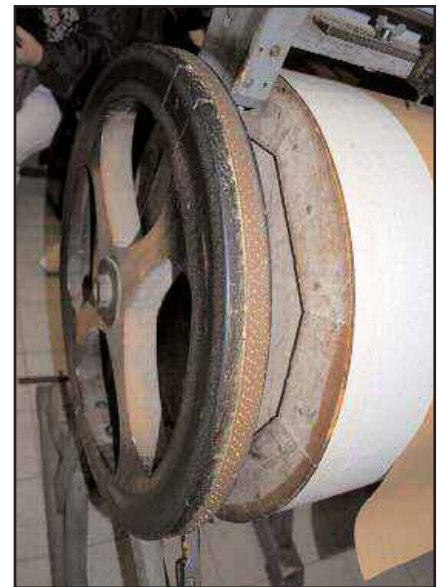
Figure 50. Arthur Prinsen's arranging drum has the tempo-setting strips on the left hand side. They are interchangeable, providing for ready arrangement of many different types of music. Author's photograph.
